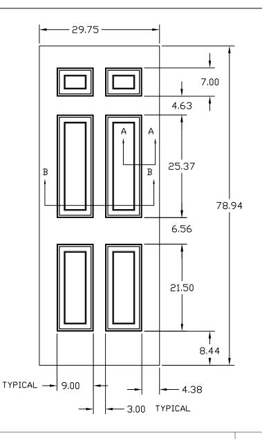
NOTE: 1/16" TOLERANCE ALLOWED FROM CENTERLINE FOR EMBOSSMENT LOCATIONS TOP TO BOTTOM AND SIDE TO SIDE.
